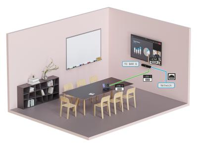
To transmit the incoming video signal from the remote station, the TC Bar can be connected directly to a display via the HDMI cable supplied.
